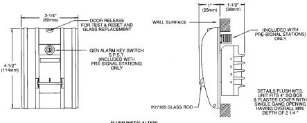
FLUSH INSTALALTION USING P-024900 STEEL BOX
